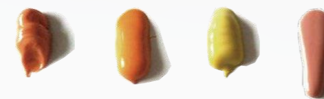
Thixotropy Test Under Static Condition
